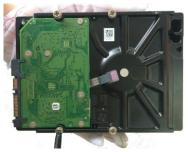
Fix the screws on the HDD, but do not be fastened.
