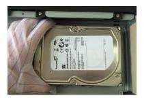
3. Put the HDD into the Device.
