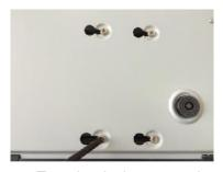
Turn the device to see the back side of it. Align the screws of the HDD with the holes on the back of the device, and then fix the screws.
