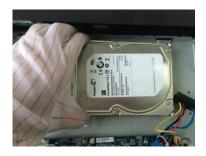
Place the HDD onto the Device.
