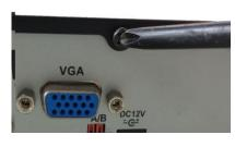
1. Remove the screws on the rear panel.
