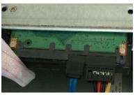
5. Use the power cable to connect HDD and mainboard.
