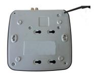
1. Remove the screws to take 2. Fix the screws on the HDD off the cover.
