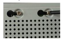
4. Turn the device to see the back side of it. Align the screws of the HDD with the holes on the back of the
