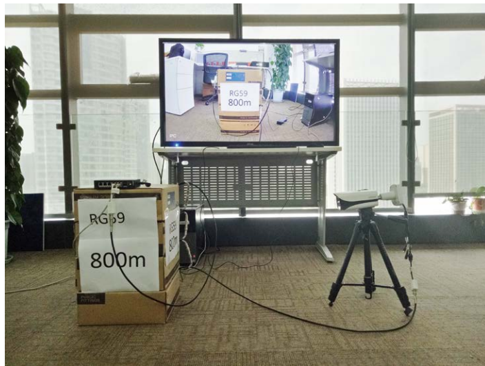
Test of 800m transmission over RG59 cable
